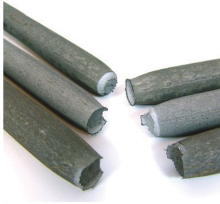
FIGURE 3.12 Cup-and-cone failure surfaces.
