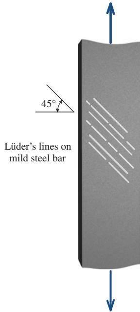
FIGURE 15.5 Lüder's lines on a ductile tension test specimen.
