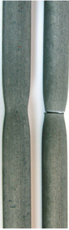
FIGURE 3.11 Necking in a ductile metal specimen.
