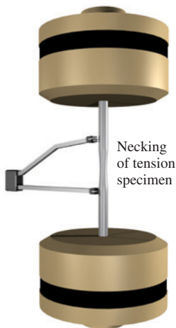
FIGURE 3.10 Necking in tension specimen.
