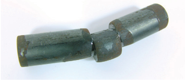
FIGURE 1.4 Double shear failure in a pin specimen.
