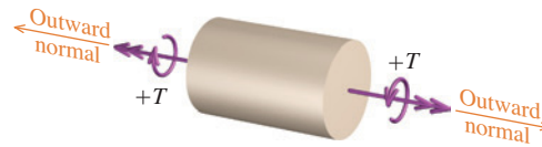
FIGURE 6.11 Sign convention for internal torque.
