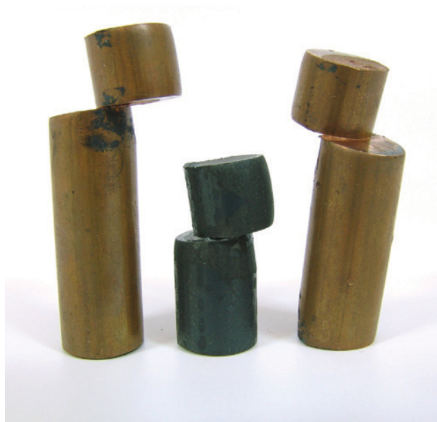
FIGURE 1.3 Single shear failure in pin specimens.
